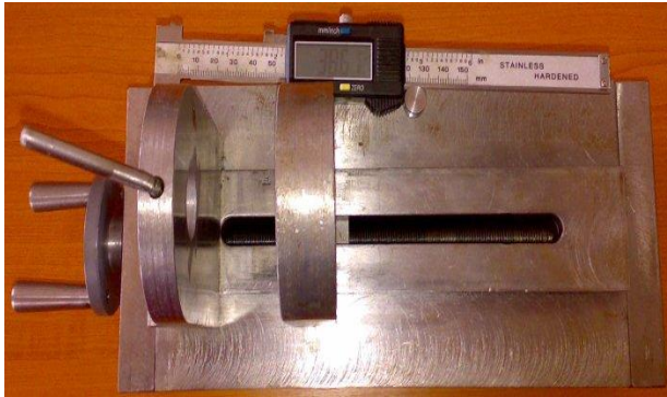
Fig. 5. Digital device for external conicity measurements (upper view)
